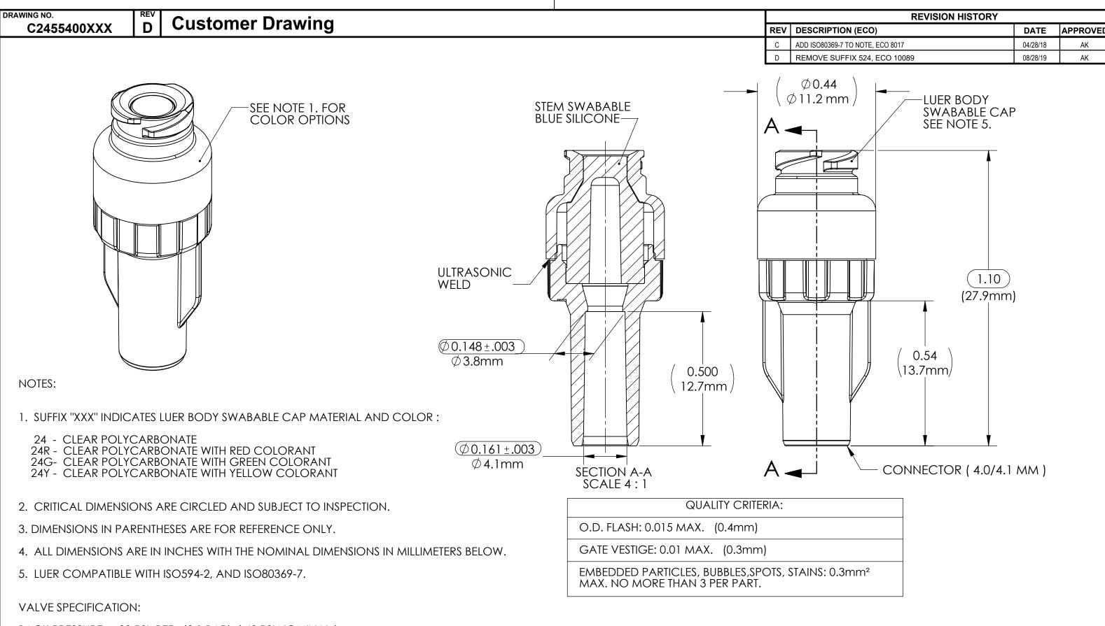
BACK PRESSURE: > 30 PSI, REF. (2.1 BAR). (40 PSI NOMINAL). BIOCOMPATABILITY: PASSES ISO 10993, PART 1.
